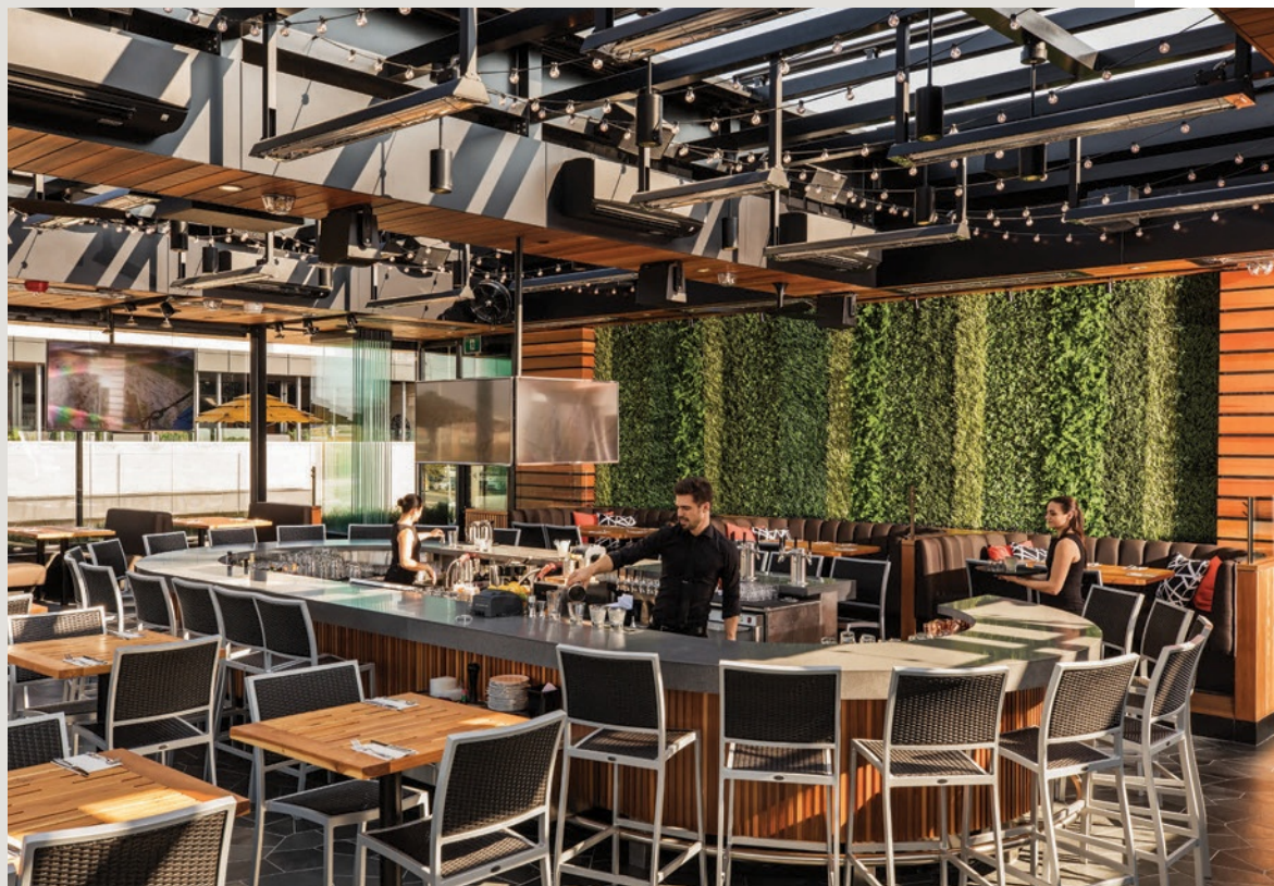
Guests can escape harsh Canadian winters into a bright and sunny space at the Cactus Club Café in the Toronto area. Assembledge+ used a combination of overhead heating arrays, fully operable slide-and-stack glass windscreens, and a retractable canopy system to accomplish this goal. Photos: Michael Weschler, courtesy Assembledge+
